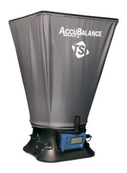
**AccuBalance Air Capture Hoods** measure air volume flowing through registers, diffusers and grilles. Weighing just 3.5 kg, these air capture hoods are easy to carry, lift and use. Simply hold the AccuBalance up to a diffuser or grille and read direct supply or exhaust airflow on the large digital display.
