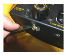
Using a 7/8" (5/8" for the CR700E) socket, loosen and remove the suctioninlet fitting and inspect the suction filter. A clogged filter will slow recovery rates. Clean with degreaser, dry and refit or replace. Replace the suction fitting 'O'-ring if mechanically damaged.
